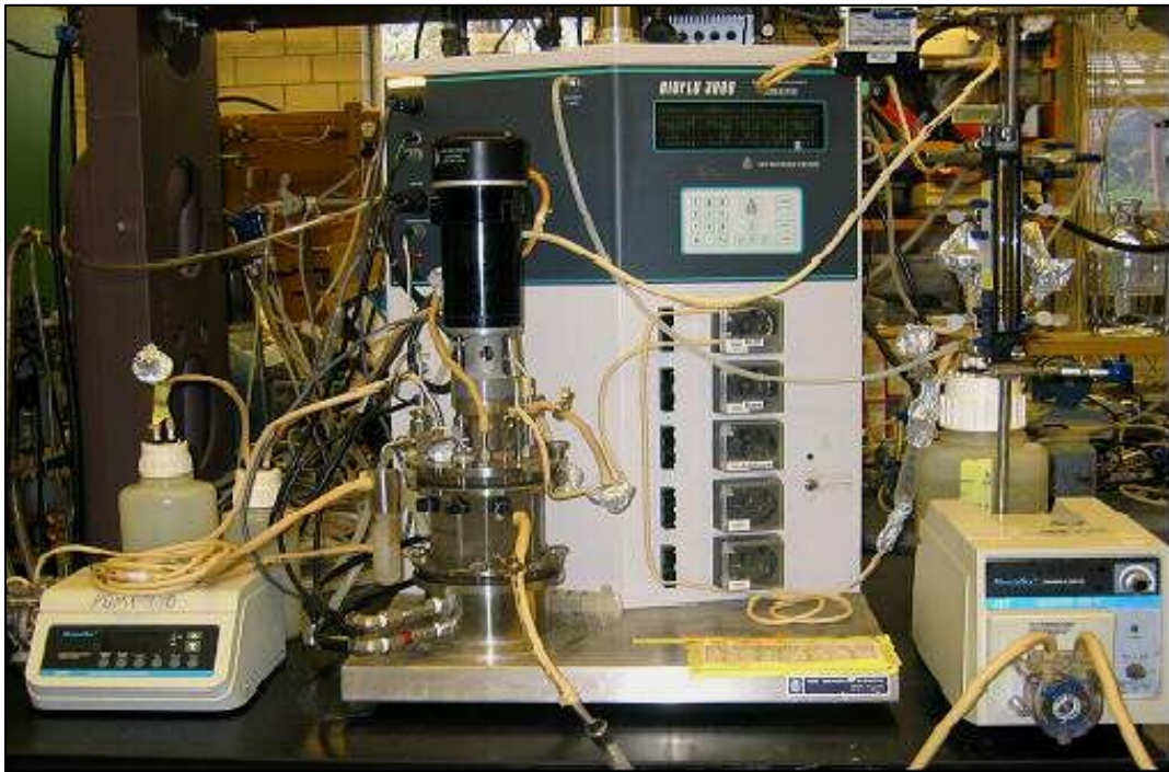
Figure A.1 Experimental set up of PCS biofilm continuous-reactor
